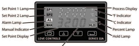
The decimal point flashes when Self-Tune is operating. Keys are illuminated when pressed. Key functions are as follows:
