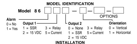
Mount the instrument in a location that will not be subject to excessive temperature, shock, or vibration. All models are designed for mounting in an enclosed panel.
