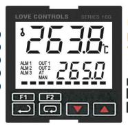
Upper display: Process Value (PV) Lower display: Set point value (SV) °C/°F: Celsius or Fahrenheit ===: Output % meter
