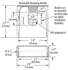
$^{\ast}\,$  Terminal block may extend up to 1/8" over the height dimensions shown.
