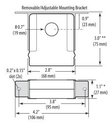
\* Terminal block may extend up to 1/8" over the height dimensions shown.
