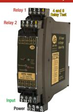
Wire terminal torque 0.5Nm to 0.6Nm (4.4 to 5.3 in-lbs)
