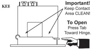
Silicone grease is factory applied on the mating surfaces to prevent rust and improve performance. Be careful not to allow grit or dirt onto the grease in the contact area. Operation can be impaired if the mating surfaces do not have good contact. Check visually before closing.
