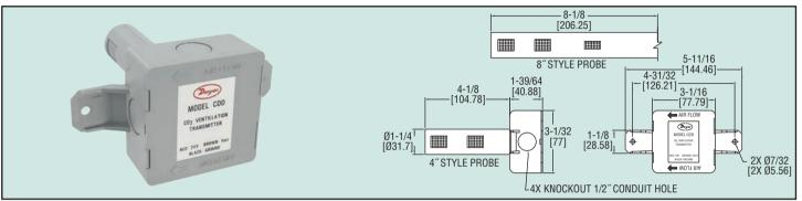
The Model CDD Duct Mount Carbon Dioxide Transmitter monitors the occupancy in a room by detecting the concentration of carbon dioxide in the return air duct. The non-dispersive infrared sensing technology automatically updates the calibration of the transmitter using a proprietary logic feature which limits the amount of error due to drift. The Model CDD can measure up to 2000 PPM in duct air flows less than 1500 FPM.
