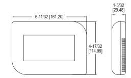
The Model TLVT1 Digital Touch Screen Programmable Thermostat with Heat Pump Control simplifies controlling indoor temperatures in commercial and residential buildings. A large easy to read LCD display shows the current temperature, set point, as well as time and day of the week.
