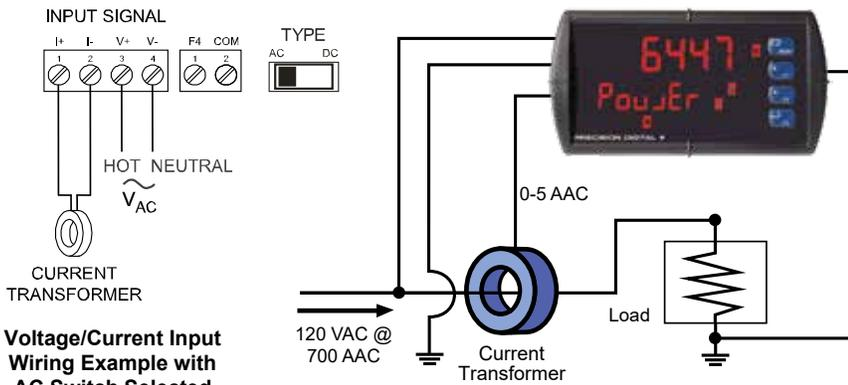
Voltage/Current Input Wiring Example with AC Switch Selected
