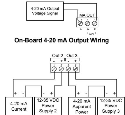
On-Board 4-20 mA Output Wiring
