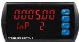
The PROVU is prompting for the value for Input 2 and displaying the default value of 5.00 A. The "5" in 5.00 is brighter than the rest of the digits indicating that it is the number that will be changed by the Up and Right arrows.
