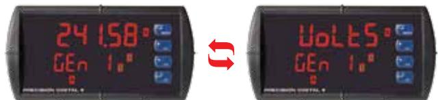
Upper line toggles between 241.58 and Volts and the lower line displays Gen 1
