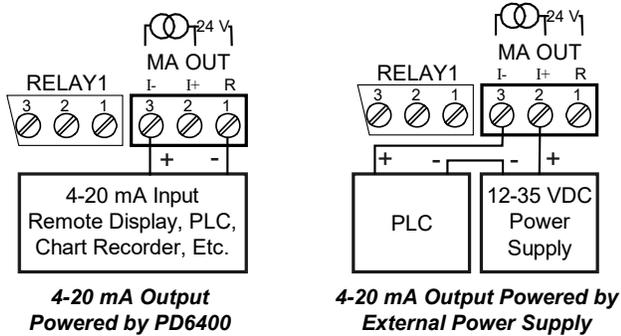
The internal 24 VDC power supply powering the analog output may be used to power other devices, if the analog output is not used. The I+ terminal is the +24 V and the R terminal is the return.
