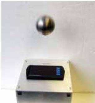
Not only does the PROVU's front panel UL Type 4X approval indicate it is waterproof, but it also indicates it is rugged. Part of the UL Type 4X test is to drop a 2 inch solid stainless steel ball from 8 feet on top of the meter's faceplate.
