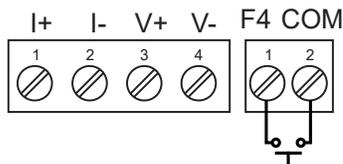
The F4 terminal is particularly useful for wiring up a remote switch to reset the relays as shown here:
