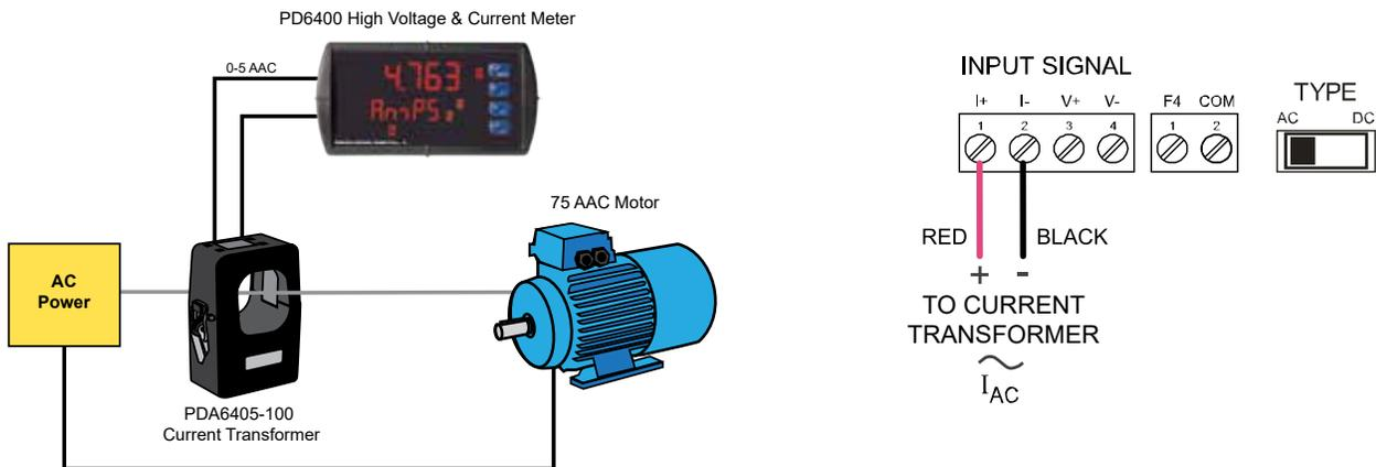
Measuring Current with PDA6405-100 Current Transformer and PD6400 digital panel meter.
