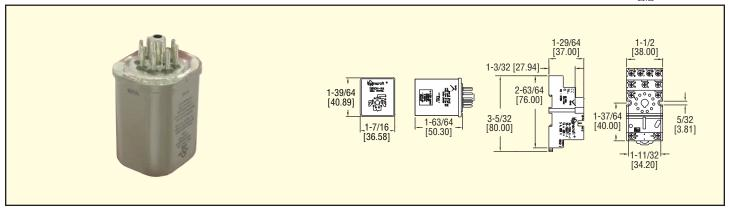
The Series 750H Hermetically Sealed Electromechanical Relay is designed to be used in Class I Division 2 hazardous area locations. Gold flashed contacts provide protection against oxidation in low current / voltage applications. 8-pin and 11-pin sockets are available to allow quick and easy installation for both surface and DIN rail mounting.
