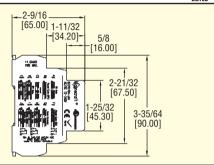
The Series 820 DIN Rail Mountable Time Delay Relays can be configured in accordance with 10 different timing functions. Bright red and green LED's indicate whether the input has been triggered and if the output is active. For greater accuracy, there are 10 time scales and a fine adjustment potentiometer that allows adjustment down to 0.1 seconds. Integral mounting ears allow the Series 820 to mount directly to a DIN rail.
