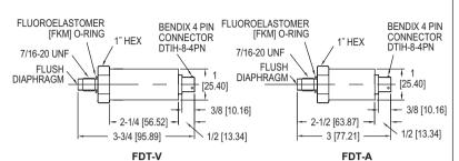
The Series FDT Flush Diaphragm Transmitter is designed for highly cyclical conditions. Flush sensor feature prevents any potential inaccuracies due to build-up or blockage which is a typical problem found in most non-flush transmitter sensors.
