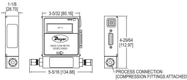
The Series GFM2 Gas Mass Flow Meter is an ideal choice for the measurement of flow rates of a wide variety of gases. Unit can be calibrated for a variety of gases with user selectable 0 to 5 VDC or 4 to 20 mA and two relay outputs and programmable totalizer that indicates total gas quantity.
