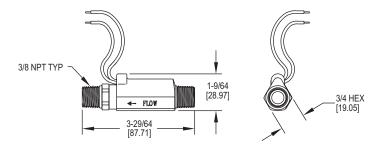
The Series P8 High Pressure Brass Flow Switch is ideal for high in-line pressures. Set points range from 0.25 to 2.0 GPM for liquid flow.
