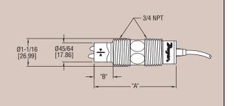
The Series TDS Thermal Dispersion Flow Switch offers solid state flow detection of non-coating liquids for pump and process protection. SPDT output allows for interfacing with remote PLC or relay control device. The adjustable switch point is factory calibrated at 0.2 fps with LED indication of flow and calibration status. Units feature selectable NO or NC operation and are not damaged by overranging flow velocities.
