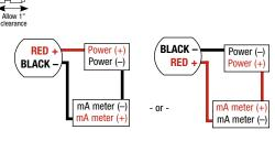
If the 4-20 mA analog output is not required, the transmitter will function as a low voltage powered temperature indicator when connected to any 8 to 32 VDC power supply. Connect the loop (+) supply to the RED lead and the loop (-) supply to the BLACK lead.
